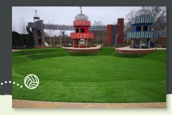
In March, we were asked back by Hampton Court Palace near Richmond on Thames to carry out some refurbishment works on their Magic Garden play area, which covers a total size of  $550m^2$ . The process involved the uplift and removal of the existing surfacing and shock pad, the supply and installation of a Playrite 10mm shock pad and then TigerTurf Finesse Deluxe synthetic turf on top.
